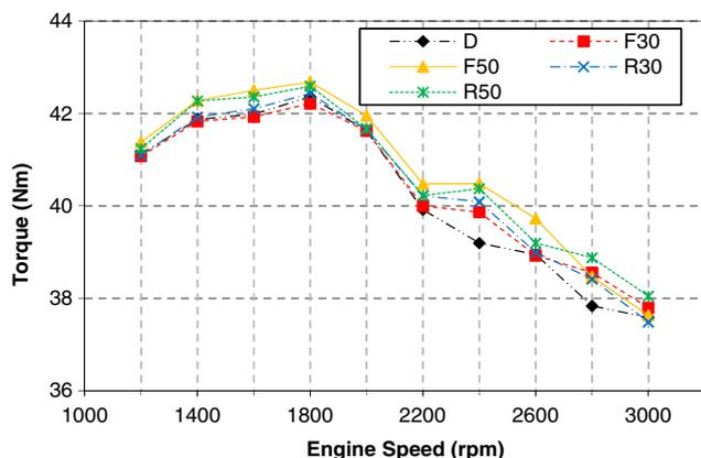
**Figure 3.** Comparison of torque between diesel and blends with metal-based additives. [Color figure can be viewed at [wileyonlinelibrary.com](http://wileyonlinelibrary.com)]
