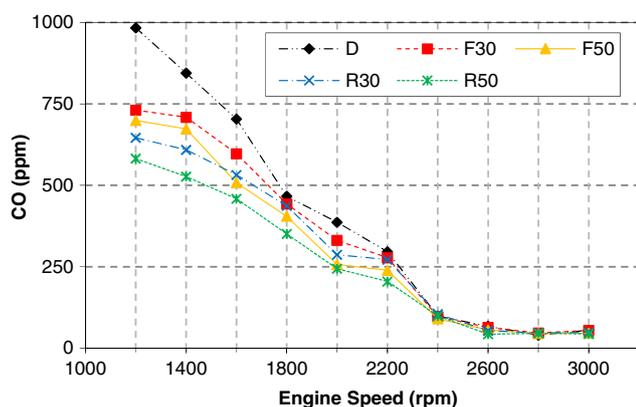
**Figure 6.** Comparison of CO between diesel and blends with metal-based additives. [Color figure can be viewed at [wileyonlinelibrary.com](http://wileyonlinelibrary.com)]
