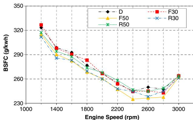
**Figure 5.** Comparison of break specific fuel consumption between diesel and blends with metal-based additives. [Color figure can be viewed at [wileyonlinelibrary.com](http://wileyonlinelibrary.com)]
