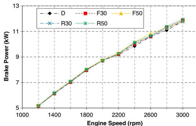
**Figure 4.** Comparison of power between diesel and blends with metal-based additives. [Color figure can be viewed at [wileyonlinelibrary.com](http://wileyonlinelibrary.com)]
