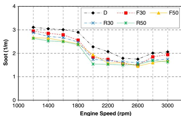
**Figure 8.** Comparison of Soot between diesel and blends with metal-based additives. [Color figure can be viewed at [wileyonlinelibrary.com](http://wileyonlinelibrary.com)]
