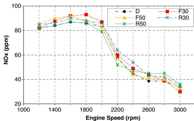
**Figure 7.** Comparison of NO<sub>x</sub> between diesel and blends with metal-based additives. [Color figure can be viewed at [wileyonlinelibrary.com](http://wileyonlinelibrary.com)]
