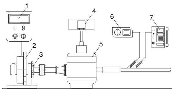
**Figure 2.** Schematic view of test bench (1: panel, 2: hydraulic dynamometer, 3: magnetic pick-up, 4: fuel tank, 5: engine, 6: sootmeter, 7: gas analyzer).
