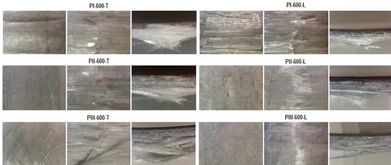
Figure 7. Optical views of composite structures after bending test (bending direction-top surface(a), reverse of bending direction-bottom surface(b), cross section(c), respectively).
