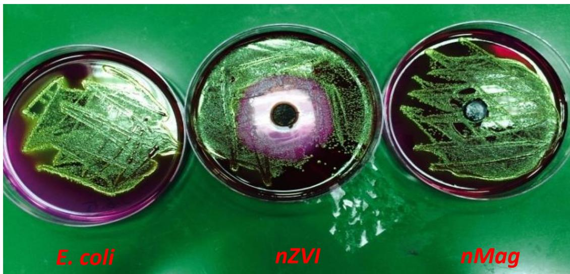
Fig. 7 (a) Control sample, (b) inhibitory zones of the nZVI pellets, (c) inhibitory zones of the nMag pellets
