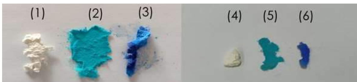
Figure 9. Raw short pulp (1), Cu-BTC deposited short pulp (2), NH 3 exposed Cu-BTC deposited short pulp (3), raw long pulp (4), Cu-BTC deposited long pulp (5), NH 3 exposed Cu-BTC deposited long pulp (6).
