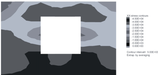
Fig. 9. Lateral Dynamic Earth Pressure Contours Leading to Highest Wall Force for Model PT-1 at 0.4 g and 3.5 Hz Excitation
