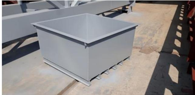
**Figure 1.** Steel sand tank used in the physical tests
