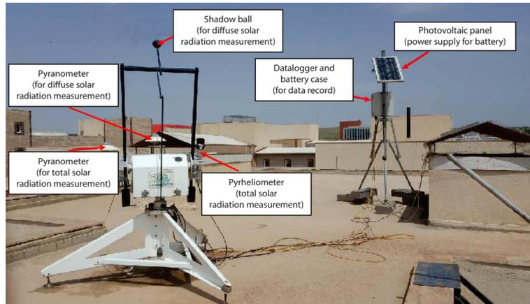
**Figure 2.** Solar radiation measurement system with solar tracking system
