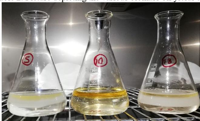
**Figure 1.** Oils from fungal biomass developed in wastewater with different C/N/P ratios (left:100/5/1; middle:100/10/1; right:100/18/1).
