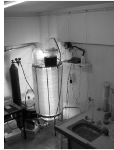
Fig. 1: Helical photobioreactor used in the experiment
