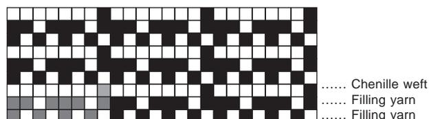
Figure 2 Weaving construction of chenille fabric.
