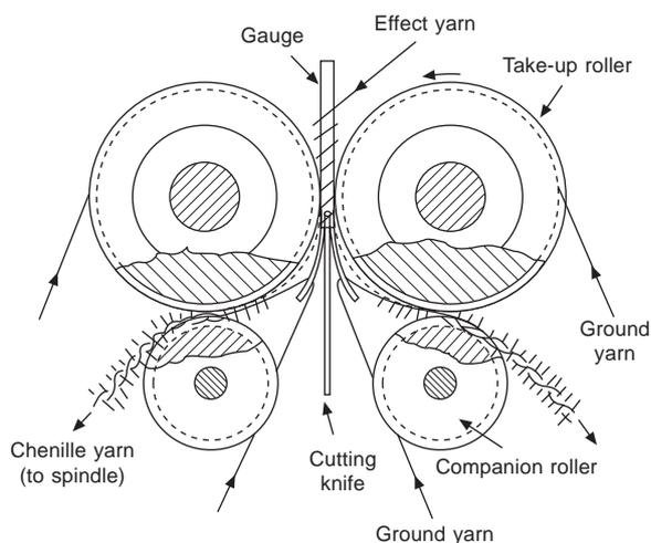
Figure 1 Chenille yarn formation in a production unit of chenille machine (Longma, 2004).
