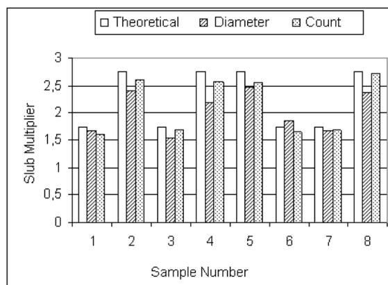
**Figure 1.** Comparison of the theoretical and measured values for slub multiplier
