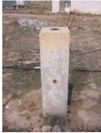
Fig. 2. One of the points established along the EDM calibration baseline (point numbered as 4)
