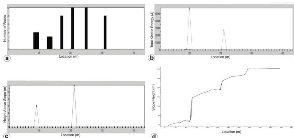
Figure 14. An example for the rockfall analyses results (profile 5) (a) runout distance (b) total kinetic energy (c) bounce height (d) the typical rockfall trajectory.
