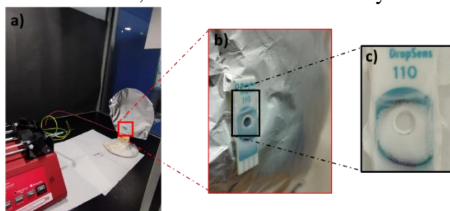
Figure 1. a) Experimental setup, b) Nanofibers on the electrode, c) Image of the fully coated working electrode.
