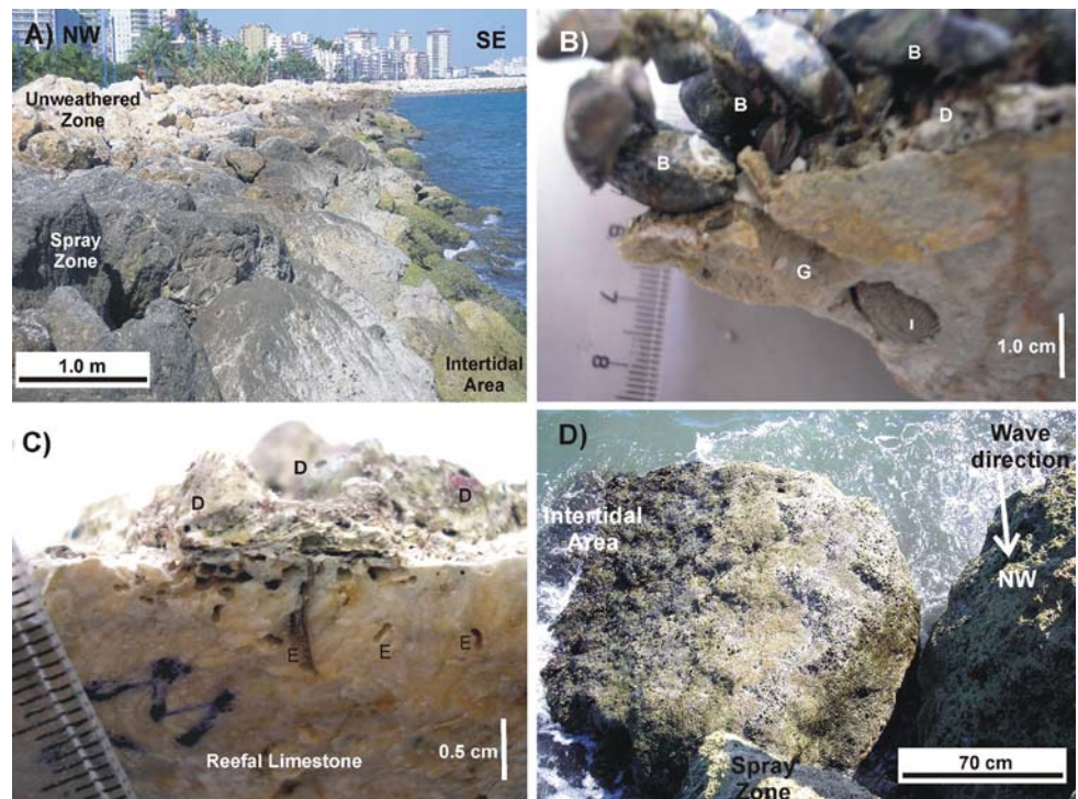
Fig. 4 a General view of the zones on the Miocene reefal limestone armourstone in the Mersin metropolitan municipality park filling area. b Bioerosive effects on samples from the subtidal zone. D , Phoronida worms; B , B. pharaonis ; G , gastrochaenolites; I , ichnofossil. c Bioerosive effects on samples from the intertidal zone; D , Phoronida worms, E , endolithes. d Field view of the intertidal zone and spray zone. Phoronida worm colonies whiten towards the upward area in the intertidal zone under the effect of atmospheric condition
