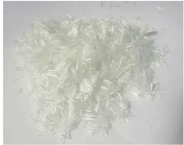
FIG. 1. Representative image of as-received state of the glass fiber waste. [Color figure can be viewed at wileyonlinelibrary.com ]
