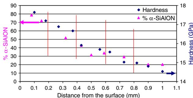
**Fig. 2.** Change in  $\alpha$ -SiAlON fraction and hardness measurements of sintered functionally graded material-B, throughout the thickness of the sample (expected interface positions are shown in the figure, and the x-axis was normalized to 1).
