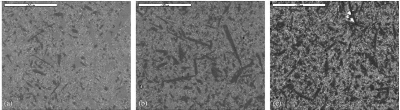
Fig. 3. BE-SEM images of functionally graded material-B (a) rich in  $\alpha$ -SiAlON content, (b) intermediate region, (c) rich in  $\beta$ -SiAlON content.
