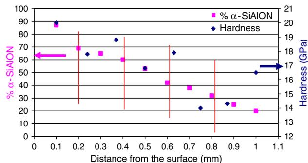
**Fig. 1.** Change in  $\alpha$ -SiAlON fraction and hardness measurements of sintered functionally graded material-A, throughout the thickness of the sample (expected interface positions are shown in the figure, and the x-axis was normalized to 1).
