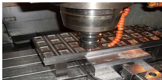
Figure 1. CNC pocket milling process [3]
