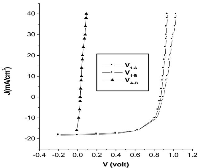
Fig. 4. J-V characteristics under illumination for a device (cell 1) with three voltage measurement cases. Parameters are given in Table 1.
