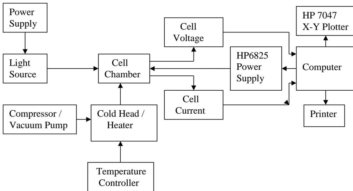
Fig. 1. Experimental set-up for measuring J-V characteristics.
