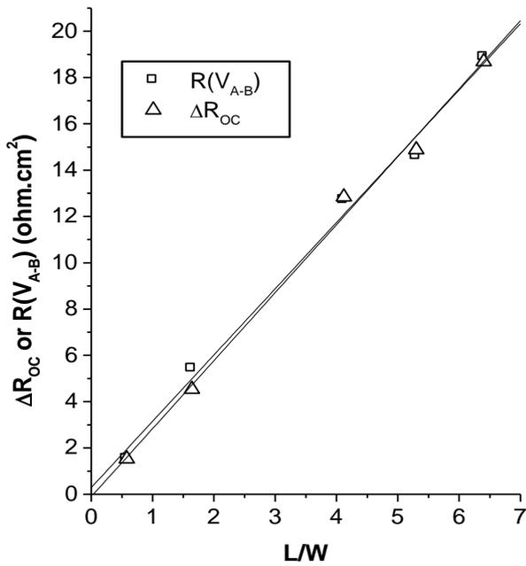
Fig. 6. Calculated resistance from both two methods vs  $L/W$  for row of cells on AFG  $\text{SnO}_2$ . The slope and intercept give the  $\text{SnO}_2$  sheet resistance and TCO/p contact resistance respectively.
