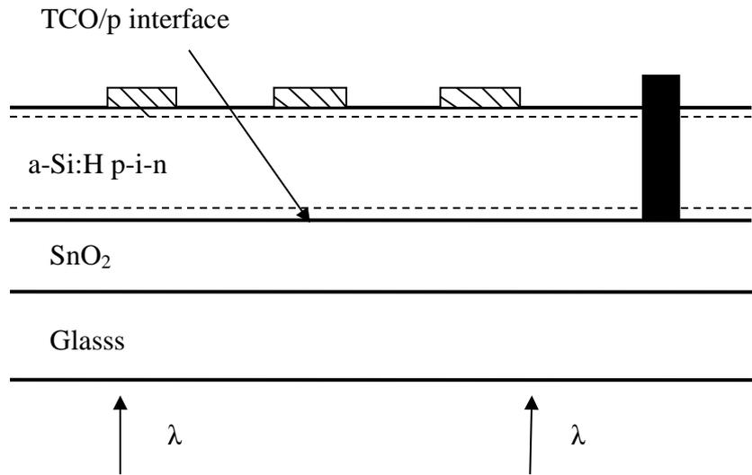
Fig. 2. Side view of row of a-Si:H p-i-n devices.
