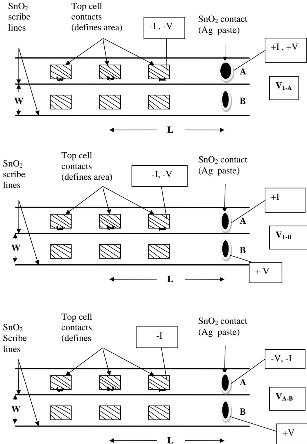
Fig. 3. Top view of row of a-Si:H p-i-n devices (1-2-3) on scribed SnO<sub>2</sub> strips with contacts labeled A and B. Current flow is established in p-i-n solar cell 1 between 1 and A while potential is measured between 1 and A, 1 and B, or A and B. SnO<sub>2</sub> strip B is floating at the same voltage as the p-layer over strip A.
