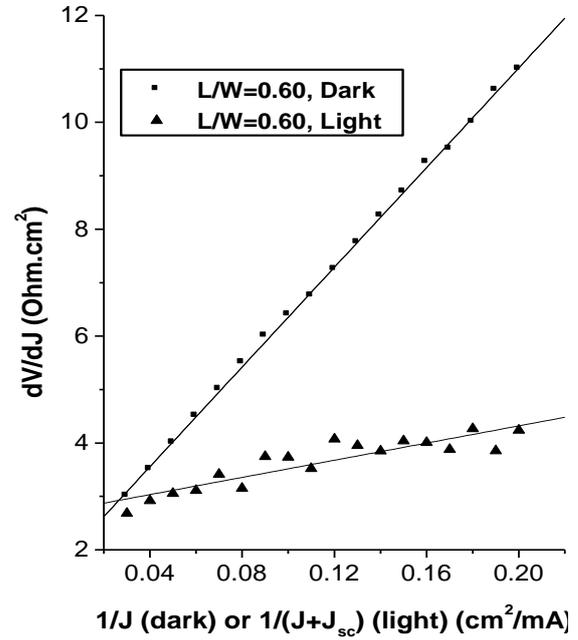
Fig. 7.  $dV/dJ$  versus  $1/J$  or  $1/(J+J_{sc})$  in the dark and under illumination respectively. The short-circuit current density,  $J_{sc} = 12.6 \text{ mA/cm}^2$ , the open-circuit voltage,  $V_{OC} = 0.88 \text{ volt}$ .
