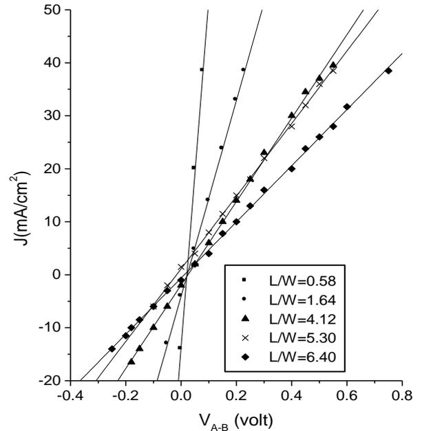
Fig. 5. J-V measurements for five devices with varying  $L/W$  on the same TCO strip A. The potential was measured across the adjacent strips A and B.
