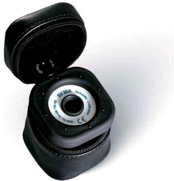
Figure 2. SV 30A Acoustic Calibrator (Svantek, Poland).
