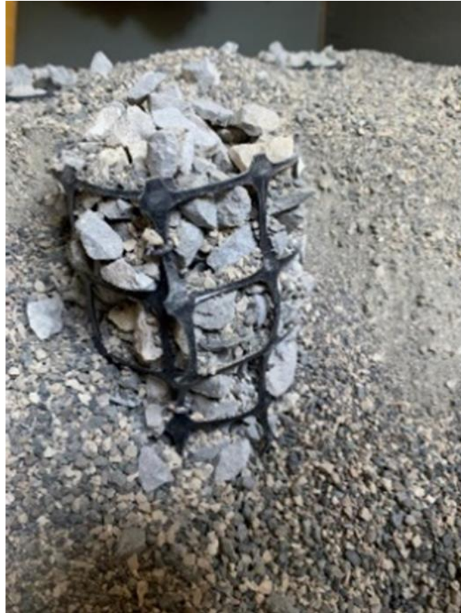
Figure 3. The bulging effect in geogrid-wrapped stone columns
