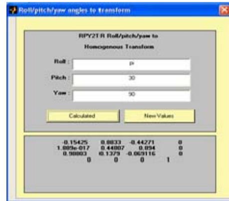
Figure 3. The screen shot of the GUI window for rpy2tr Command in GRAK
